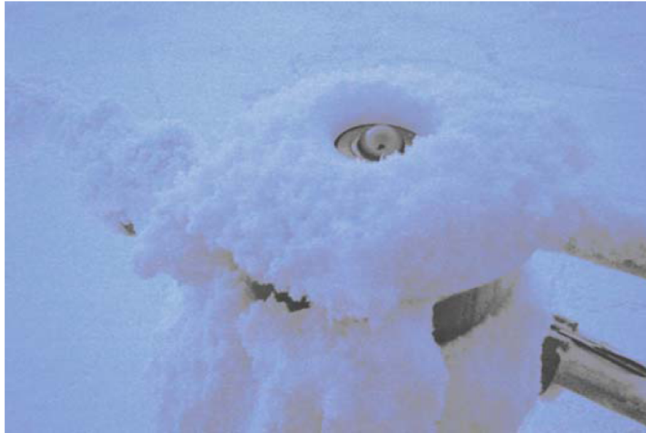
Fig. 7: Example of extreme riming on a heated and ventilated Kipp and Zonen pyranometer at Eureka, Ellesmere Island in late October 2009. Although the dome isn't rimed, the build-up around the dome will degrade the radiation measurement.
