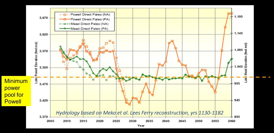
Modeled Powell (orange) and Mead (green) year-end elevations, under No Action (dashed) and Preferred Alternative (solid), using trace starting in AD 1130.
