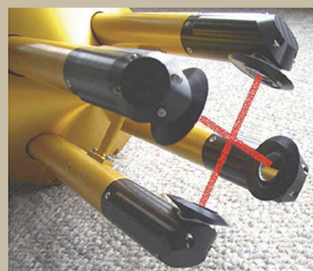
Fig. 1(b) 2D-Stereo (or 2DS probe) (Source: Lawson et al, 2006: J. Atmos. And Oceanic Tech.)
