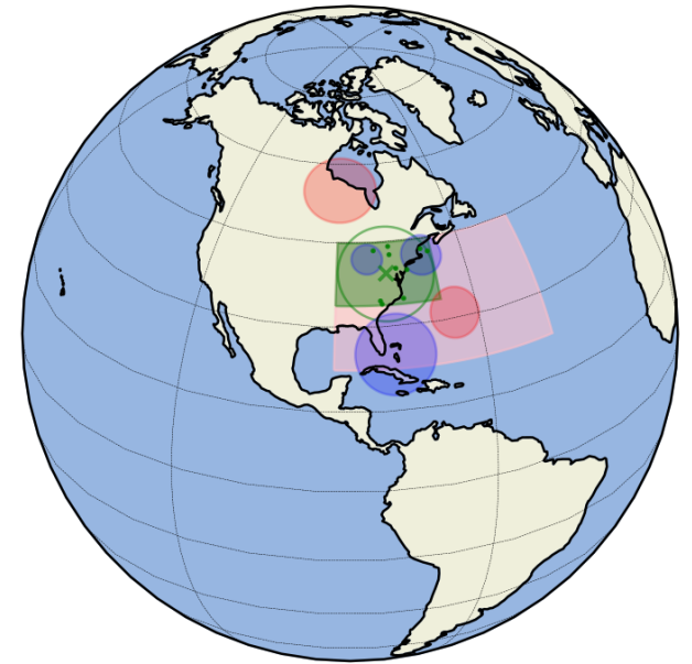
Figure A.1: Horizontal schematic of Octree application on spherical coordinate. The pink box is one of the three-time-divided boxes, which is 45 degrees in longitude and 22.5 degrees in latitude. The green box is one of the four-time-divided boxes. The green cross, dots, and circle show the center of the green box (at 39.375°N 78.75°W), hypothetical observations in the green box, and the radius of the box after adding the observations (approximately 943 km), respectively. Note that the observations (green dots) exist only in the intersection of the green box and circle. Queries like the blue (red) circles intersect (does not intersect) with the green circle and may (may not) find observations in the green box.
