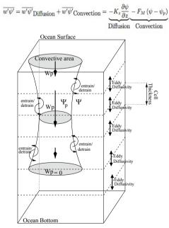
Schematic representation of a convective plume in a single grid-cell
