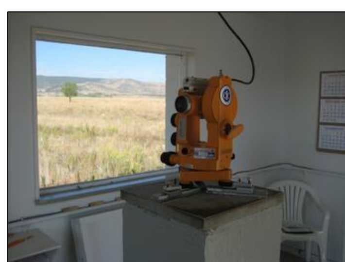
Zeiss Jena O10B Theodolite for making absolute measurements at Boulder magnetic observatory
