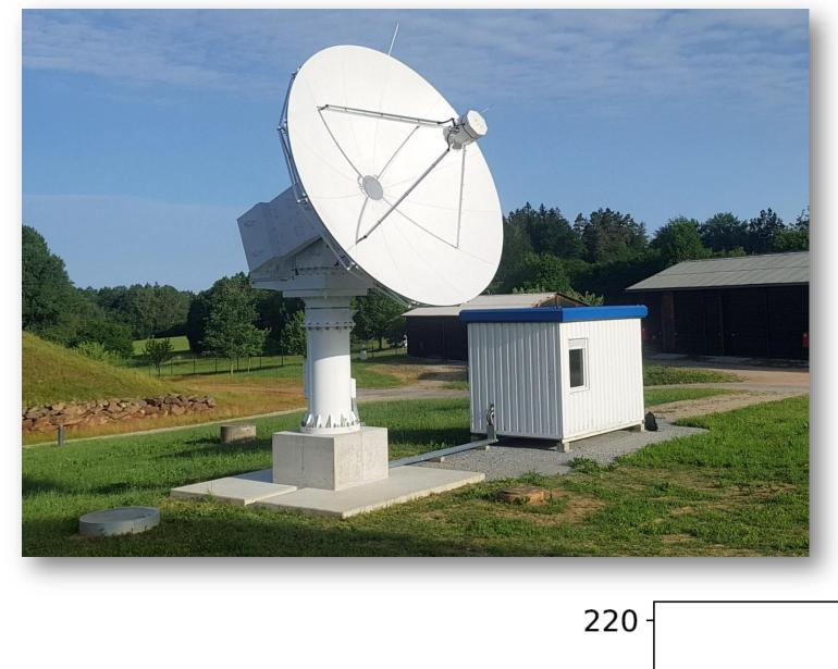
The Solar Flux Telescope shown on the left is used to directly observe the solar radio flux per unit frequency in the radio wave range. The telescope has an aperture of five meters. Among other frequencies, observations are made at 2800 MHz to determine the F10.7 index (corresponding to a wavelength of 10.7 cm). On the lower right you see a first test measurement recorded during the perihelion of the Parker Soral Probe.
