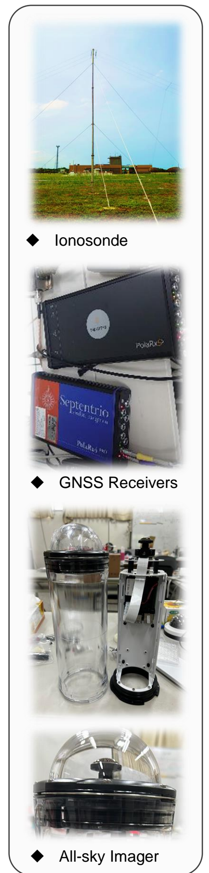
Fig. Integrated ionospheric irregularity observations via satellite (F7/C2) and ground instruments (ionosonde, GNSS receiver, and all-sky imager).
