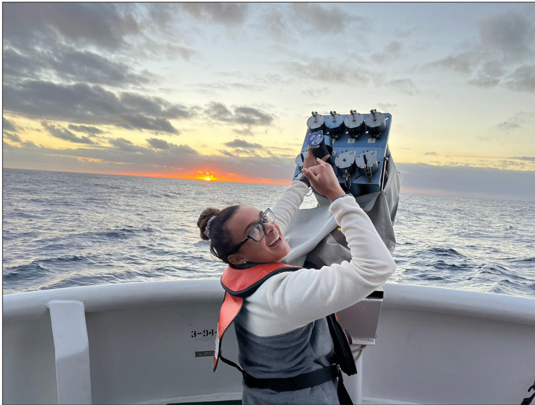
Jennifer Clifton, Explorer-in-Training, reloads an expendable bathythermograph (XBT) to collect ocean temperature data. Photo courtesy of NOAA
